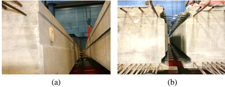
Figure 2.34: (a) Conventional shear key specimen and (b) UHPC shear key specimen [63]
