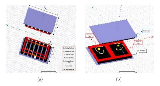
Figure 6.4: 3D-FEA model of 2 (a) DD (b) BPP Coupler
