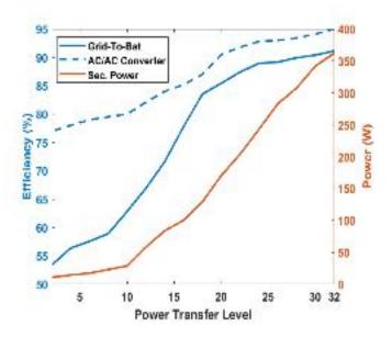
Figure 8.15: Efficiency plots at different power transfer levels
