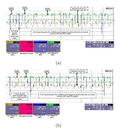
Figure 8.9: Switching signals when the multi-power level controller is set to operate in total level of 5 ( $L_{neg} = 3$  and  $L_{pos} = 2$ ) (a) Dip switches for power level selector for positive are set  $P_3P_2P_1P_0 = "0001"$  (b)Dip switches for power level selector for negative are set  $N_3N_2N_1N_0 = "0010"$
