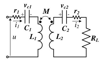
Figure 5.2: Series-compensated inductive charging system: equivalent circuit and corresponding variables.
