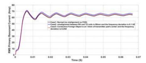
Figure 2.5: Resonant RMS current during normal conditions, misalignment and FOD maximum frequency deviation of 8Hz
