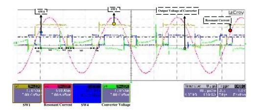
Figure 4.11: Experimental result for switching signals(SW2 and SW3), resonant current and converter output voltage when input AC voltage are positive
