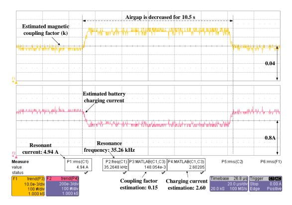
Figure 5.7: The estimated coupling factor and battery charging current while the airgap is reduced for 10.5 seconds.
