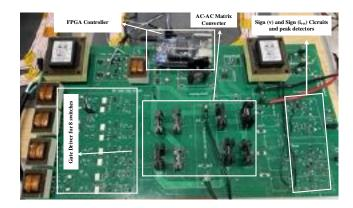
Figure 8.7: Resonant high frequency converter with FPGA-based IPT power controller
