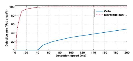
Figure 2.23: The plot of the detection area as function of detection speed for two tested foreign objects.
