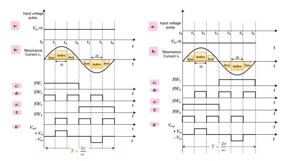
Figure 4.3: when ac supply voltage is Figure 4.4: when ac supply voltage is positive  $(V_{ac} > 0)$  negative  $(V_{ac} < 0)$
