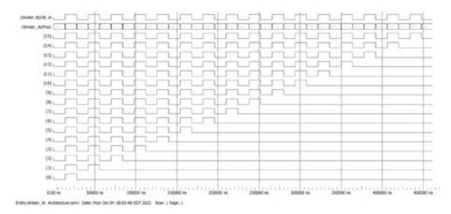
Figure 8.4: Count5(k) (k = 0 to 15) which contains the (k+1) pulses in positive half cycles
