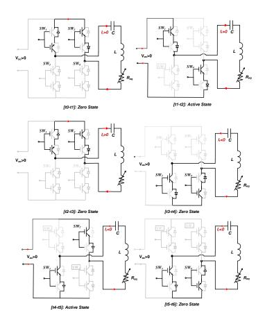
Figure 4.2: IPT's primary resonant current path for six operation modes when ac supply voltage is in positive half cycle  $(V_{ac})$
