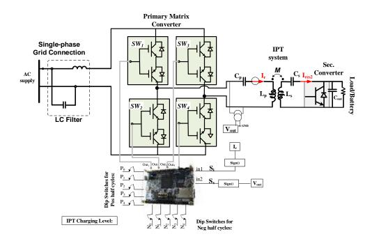
Figure 8.1: Conceptual Picture: AC-AC Matrix Converter and IPT system
