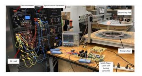
Figure 1.2: Proposed Multi-power level controller for dynamic inductive electric vehicle charging using estimated position
