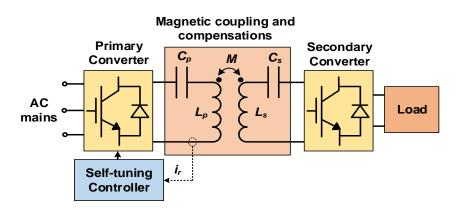
Figure 2.7: Schematic diagram of the IPT system.
