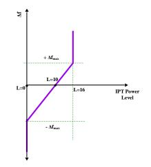
Figure 3.17: Frequency deviation VS the IPT power level number (1  $\% < SOC < 99\,\%)$
