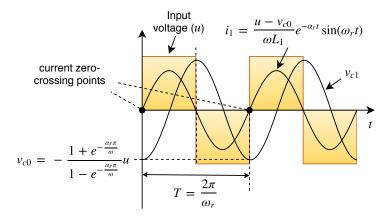
Figure 5.3: A conceptual plot of the resonant current, capacitor voltage and corresponding analytical formulations.
