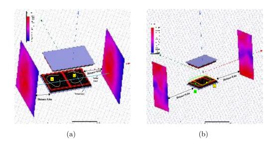
Figure 6.5: Magnetic flux density in 0.4m distance (a) BPP (b) DD Couplers
