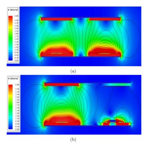
Figure 2.8: 2D FEA analysis: (a) magnetic flux density without object presence, (b) magnetic flux density with the presence of conductive object.
