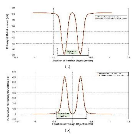
Figure 2.16: FEA analysis for aluminum and iron foreign objects(a) Primary self-inductance  $(L_P)$  distortion for two different material of FOI(b) Resonance frequency deviation for two different material of FOI.
