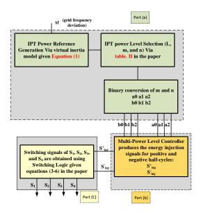
Figure 3.2: The flowchart of the virtual inertia based IPT power controller
