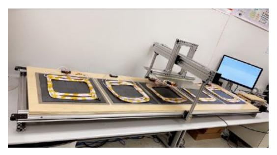
Figure 7.14: The experimental setup for dynamic IPT system which is built based on "POS-6" design values
