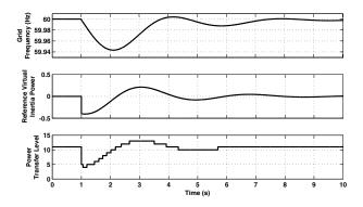
Figure 3.10: Simulation results: Grid frequency (f), power deviation $(\Delta P)$ , IPT power level
