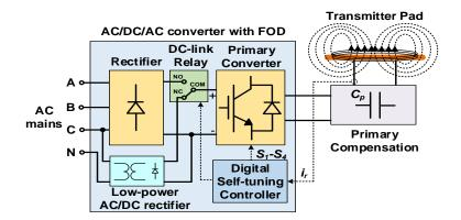
Figure 2.15: Proposed IPT system with consideration of low lower AC/DC rectifier to provide DC link for FOD purpose in the standby mode.
