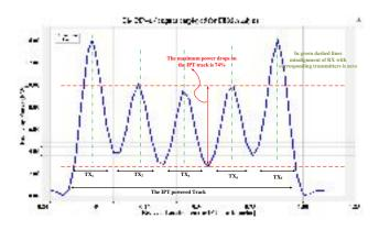
Figure 7.11: Receiver Power when IPT track is set with PSF-1
