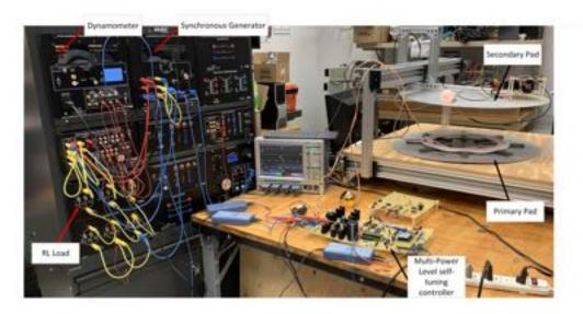
Figure 3.12: Experimental setup: Inductive Power Transfer connected to an Lab-Volt grid emulator which is comprised of synchronous generator, RL loads.
