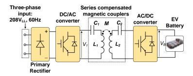
Figure 5.1: A typical Series-Series IPT system
