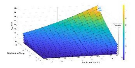
Figure 8.8: 3-d plot: output power vs energy injection in positive half cycle( $L_{pos}$ ) vs energy injection in positive half cycle( $L_{neg}$ )
