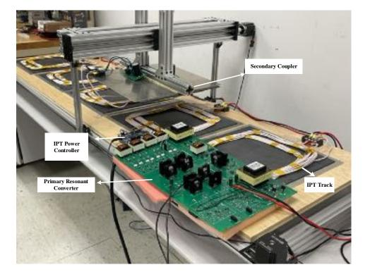
Figure 8.6: Dynamic IPT setup comprised of 5 bipolar transmitting couplers and a receiver
