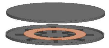
Figure 2.10: 3D electromagnetic model of IPT system.
