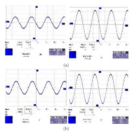
Figure 2.26: Experimental results for larger size foreign objects(a) Primary/secondary resonance currents when the new resonant frequency caused by FOI is about 36.033 kHz (b) Primary/secondary resonance currents when the new resonant frequency caused by FOI is about 37.306 kHz.
