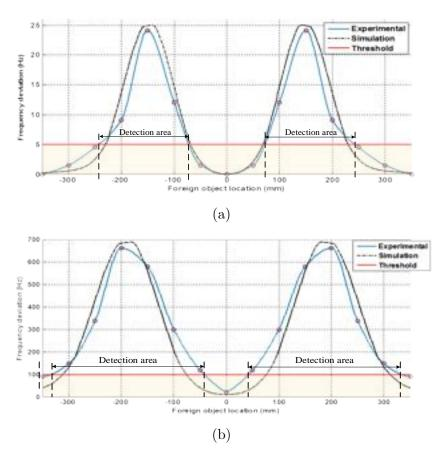
Figure 2.22: Experimental results achieved by the proposed FOD method(a) 5-cent coin (49% detection area) with 200 ms sampling time (b) Beverage can (with 82% detection area) with 10 ms sampling time.
