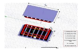
Figure 7.4: BPP 3-D FEA model with all the defined parameters
