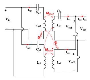
Figure 6.2: IPT systems consists of two primary couplers (TX1, and TX2) and two secondary couplers (RX1, and RX2)
