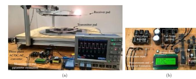
Figure 5.6: The experimental setup of the inductive charging system prototype with online parameter estimation functionality.
