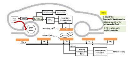
Figure 6.1: The conceptual schematic of IPT roadway-powered track for dynamic EV charging system
