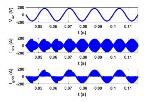
Figure 4.6: a)  $v_{ac}$  b) Resonant Current  $(I_{res})$  c) Grid Current  $(I_{grid})$
