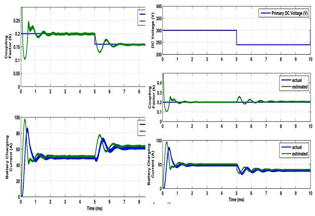
(a) 20% sudden reduction in coupling factor (b) 17% sudden reduction in primary DC voltat t = 5ms age at t = 5ms.
