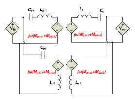
Figure 7.3: Simplified IPT circuit using FHA method
