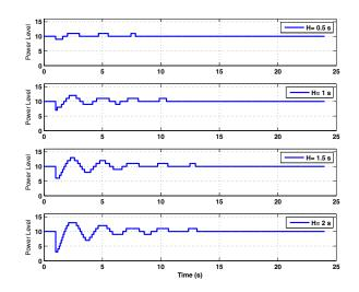
Figure 3.11: Virtual inertia response of the proposed IPT to power grid dynamics with various inertia Constants.
