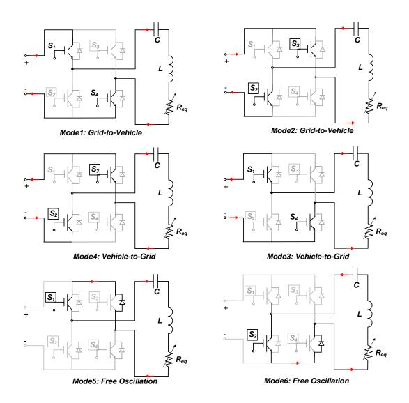
Figure 3.6: IPT's primary resonant current path for six operation modes (referring to Table 3.3)
