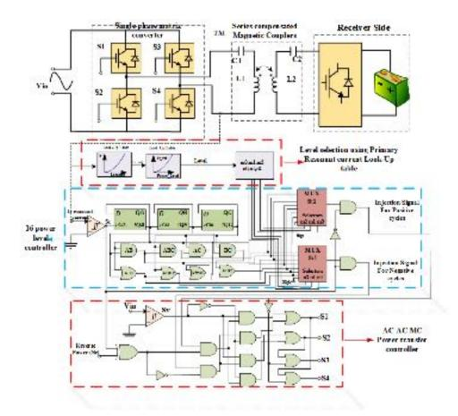
Figure 7.17: Proposed control of DWPT for matrix converter for primary current regulation according to pickup side position
