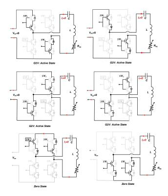
Figure 8.5: Equivalent circuit operations with active and zero states for Grid to Vehicle operational mode
