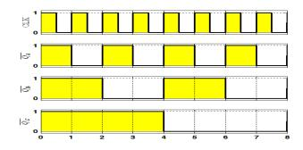
Figure 3.4: Reference CLK (used as the clock signal for the first D-type flip-flop), and inverted outputs:  $\overline{Q_A}, \overline{Q_B}, \overline{Q_C}$  of three cascaded flip-flops (see Fig. 3.3)
