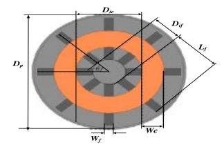
Figure 3.7: Geometrical parameter of ferrite bars, coil, and shield plate in the circular power pad
