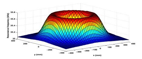
Figure 2.14: 3D plot of resonance frequency as function of foreign object location respect to primary pad center.
