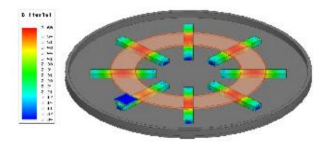
Figure 2.11: distribution of flux density on the primary pad.
