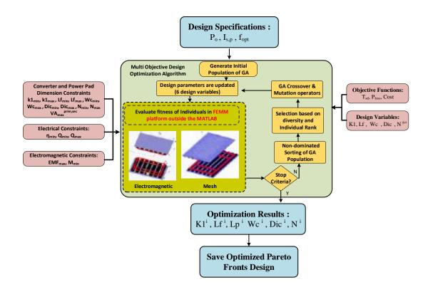
Figure 7.5: The proposed multi-objective time-harmonic algorithm using cosimulation of FEMM software and MATLAB
