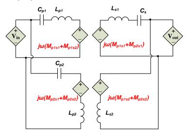
Figure 6.3: Simplified IPT circuit for double couplers configuration using FHA method
