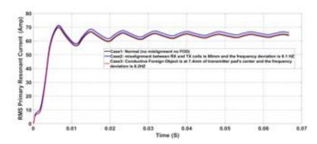
Figure 2.19: Resonant RMS current during normal conditions, misalignment and FOD maximum frequency deviation of 8Hz.
