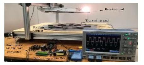
Figure 2.21: Inductive Power Transfer Experimental set-up.
