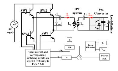
Figure 4.1: Schematic: AC-AC matrix converter for IPT system
