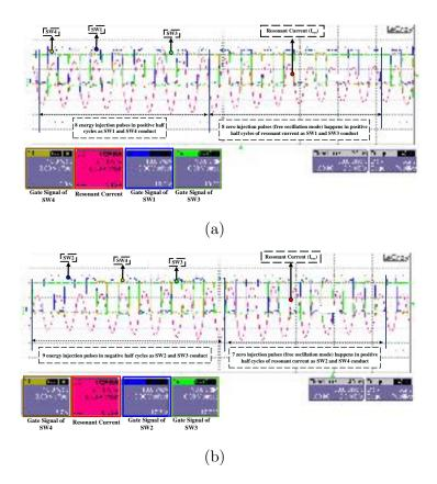
Figure 8.11: Power level controller is set to operate in total level of 17 ( $L_{neg} = 8$  and  $L_{pos} = 9$ ) (a) Power level selector for positive are set  $P_3P_2P_1P_0 = "0111"$  (b)Power level selector for negative are set  $N_3N_2N_1N_0 = "1000"$
