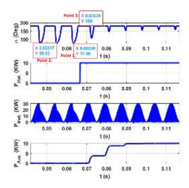
Figure 4.5: a) Converter's conduction phase  $(\alpha)$  b) reference power change  $(P_{ref})$  c) IPT's instantaneous Power  $(P_{ints.})$  d) Averaged IPT power over 60 Hz time period  $(P_{Ave.})$
