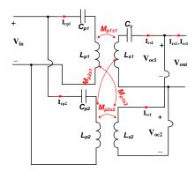
Figure 7.2: IPT systems consists of two primary couplers (TX1, and TX2) and two secondary couplers (RX1, and RX2)
