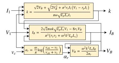
Figure 5.4: The flowchart of the developed parameter estimation method based analytical formulations.
