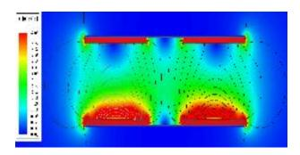
Figure 3.8: 2D-FEA Model: Magnetic plot of the IPT system
