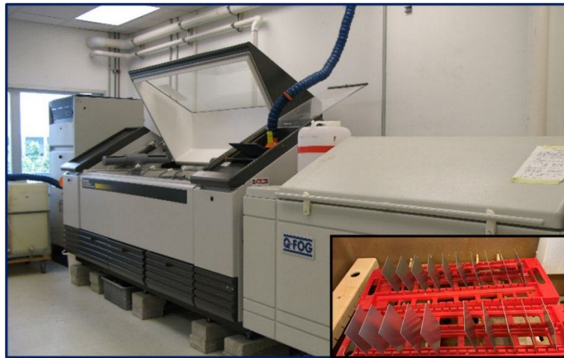
Figure 26: Photograph of Q-Fog neutral salt fog chamber and inset is examples of test panels on the polypropylene slotted support rack between 15 and 30°.
