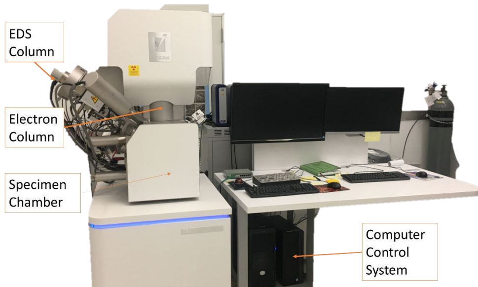
Figure 15: Schematic image of NASA KSC Scanning Electron Microscope (SEM), TESCAN FIB-SEM typical with major components labeled.
