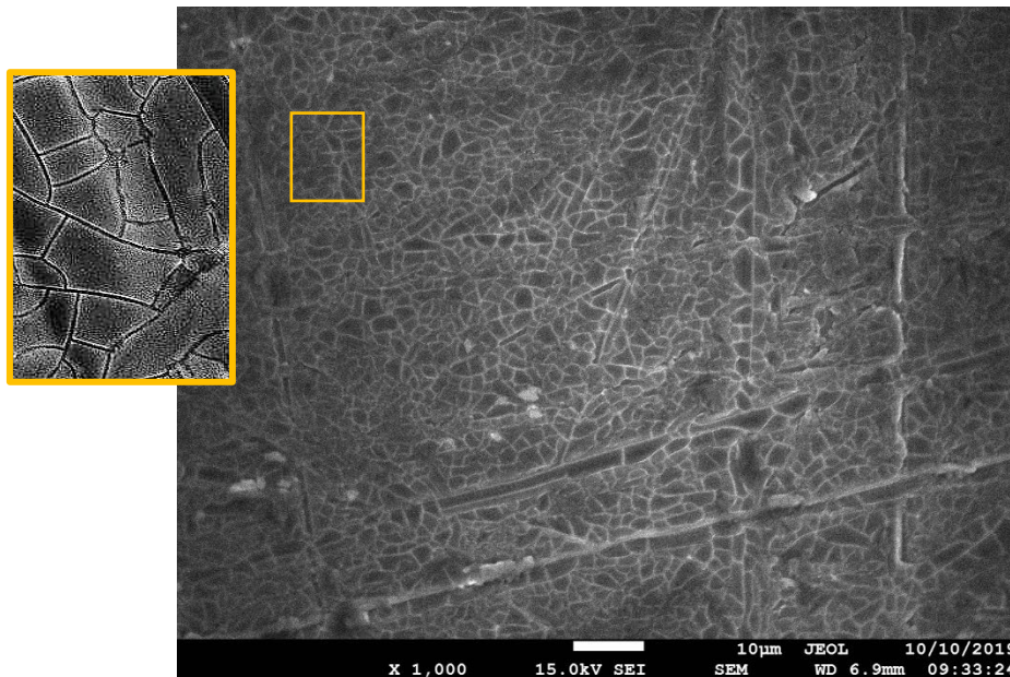
Figure 10: SEM images (magnification 1000x) of the aged CCC on Al2219, illustrating the mud-cracking surface film features. Inset picture is of 10kx magnification.
