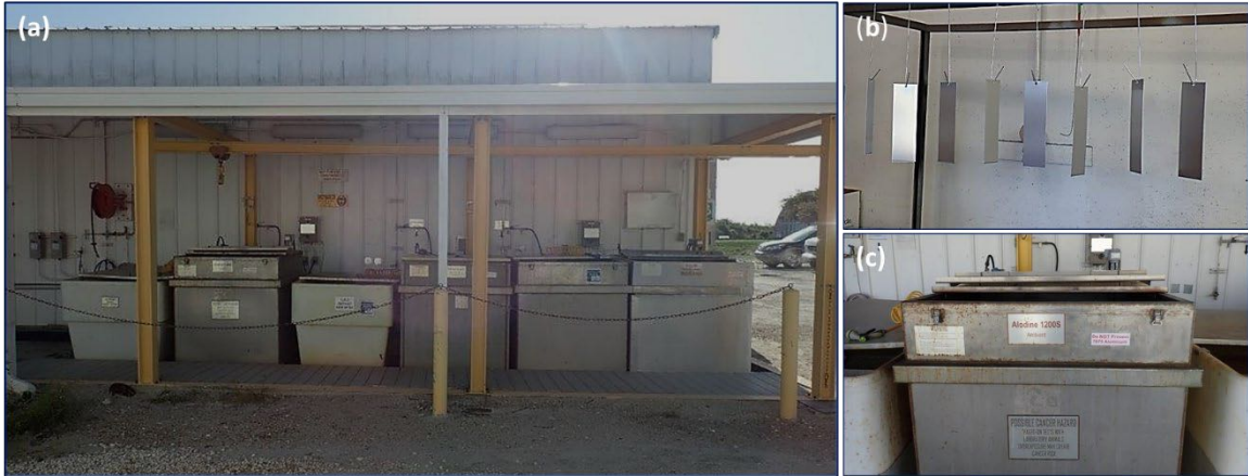
Figure 24: (a) NASA LES Machine shop chromate conversion line, (b) Al2219 samples drying after coating, and (c) chromate tank.
