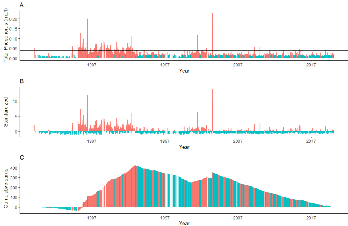
Figure 2.2: For total phosphorus, Box A depicts the values of total phosphorus in the Miami River across all sites and the black line is the EPA standard at 0.04 mg/L. Box B shows standardized values, where phosphorous values across all sites were subtracted by the average of the data set for phosphorus and divided by the standard deviation while Box C shows cumulative sums of the standardized values, showing shifts in the data as it moves below or above average. Values above average are depicted in red and below average values are depicted in blue.
