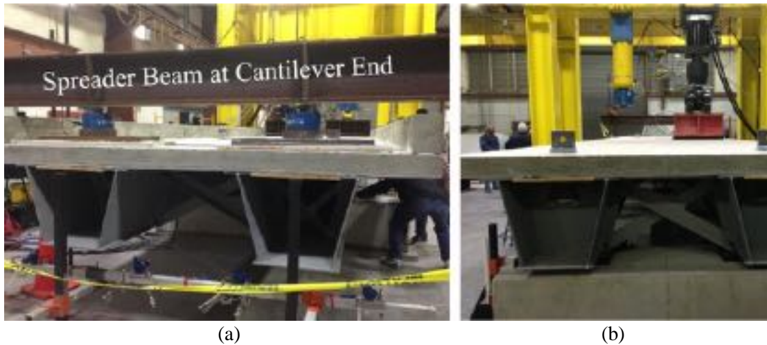
Figure 2-34. The FIU test setup: (a) View from the cantilever end; (b) View from the simply supported end.
