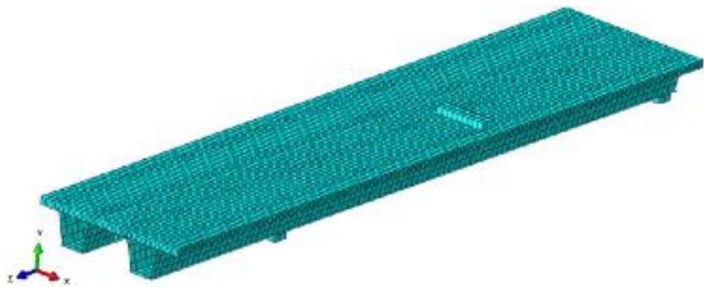
Figure 2-38. The FIU bridge FE model.
