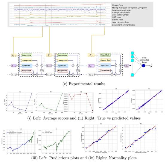
Fig. 3. Implementation of the proposed LSTM-SDM framework for S&P 500 index price prediction [12].
