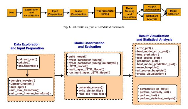
Fig. 2. Workflow analysis of LSTM-SDM functionalities.
