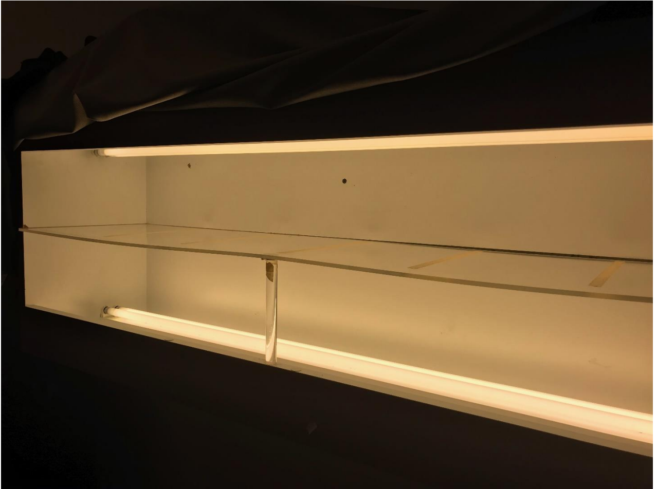
Figure 4: IROC- Houston custom bleaching box. Consists of two parallel opposed halogen bulbs with an acrylic plate to hold OSLDs
