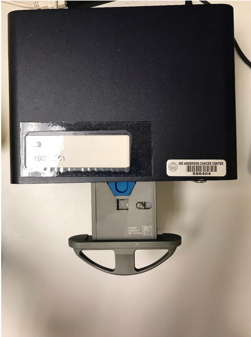
Figure 11: Top View of the Microstar II reader with the loading tray extended
