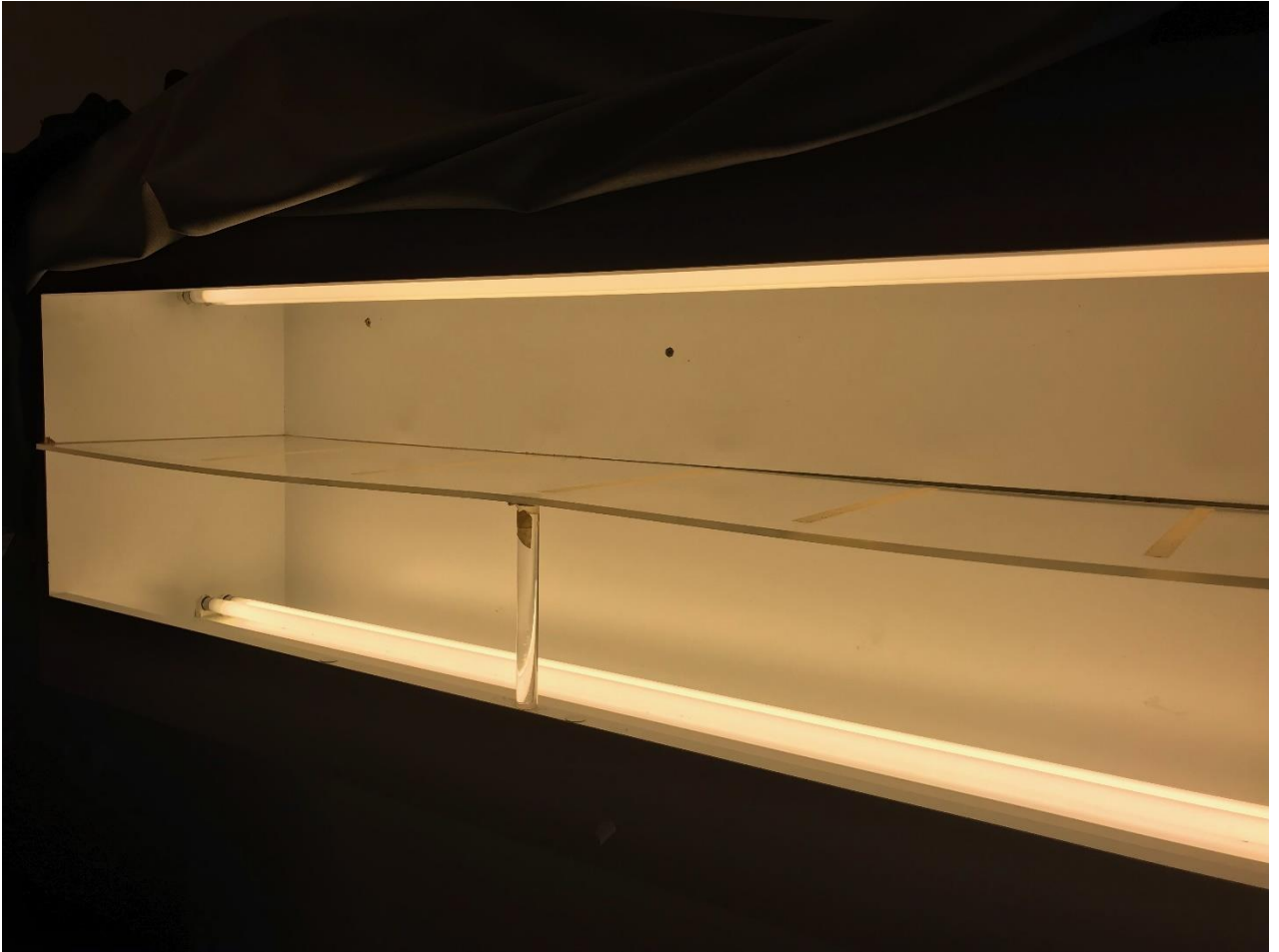
Figure 13: IROC- Houston custom bleaching box. Consists of two parallel opposed halogen bulbs with an acrylic plate to hold OSLDs
