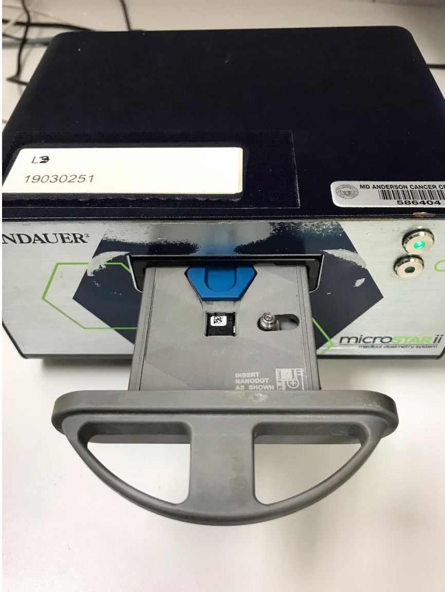
Figure 12: View of the Microstar II reader with a nanoDot OSLD inserted
