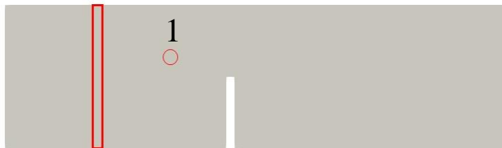
Figure 5.18 Monitor point No. 1 (Mid-point of turbulence source and building) and position of turbulence source (red square) and building.
