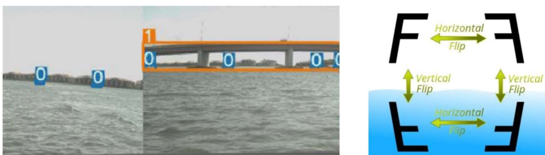
Figure 16 Augmentations. Shows a mosaic augmentation on the left and shows different flips on the right (Hasty, Horizontal Flip, 2022).
