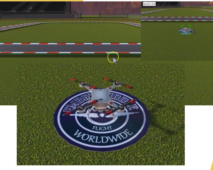
ERUPTSim was ERAU WW developed. The flight simulator (Unityengine) offers training remote pilots of drones/sUAS.
