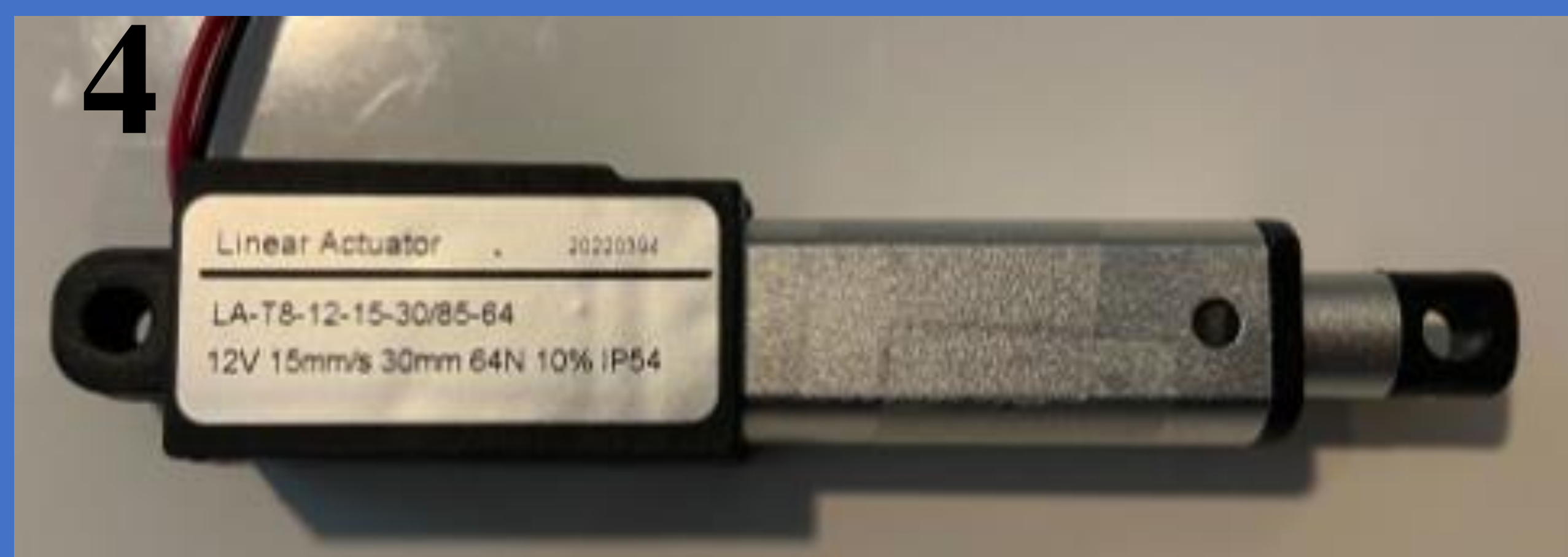
Image 4: Mini Linear Actuator used to move the plate that holds the magnet in the M.A.S. These actuators can be programmed to actuate at specific frequencies.
