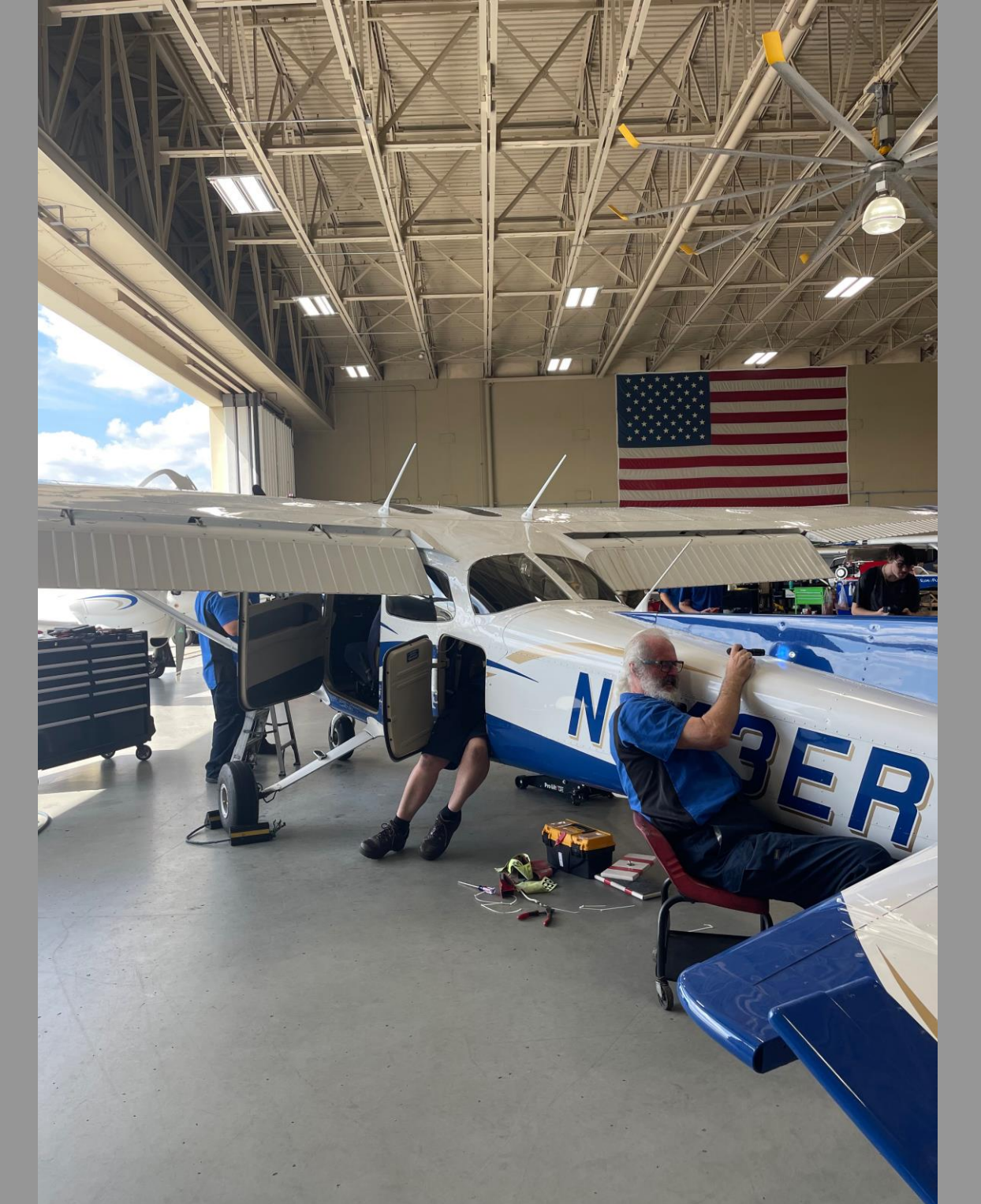
Figure 3. Additional ergonomic postural issues found during air conditioning overhaul the REBA assessment.
