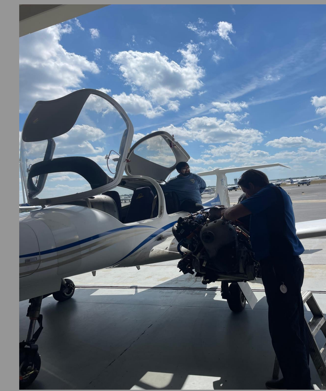
Figure 2. Demonstration of the engine maintenance process assessed by the REBA.
