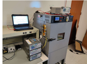
Figure 1: Image of the calibration setup in SAIL. Test Equity 115A shown on right. Left: Up to 3 Keithley 2450 source meters for simultaneous calibration.
