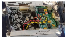
Main Payload Accelerometer Box
