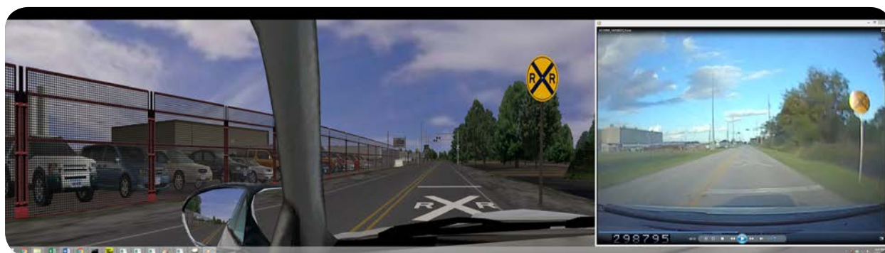
Figure. Driver Simulator (left) vs. the actual view (right) at one of the tested HRGCs
