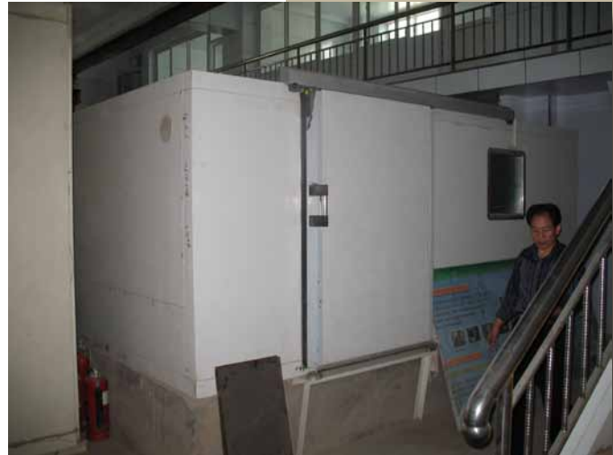
Temperature controlled research “rooms” (freezers) in CAREERI for investigating frozen embankments and their thawing.
