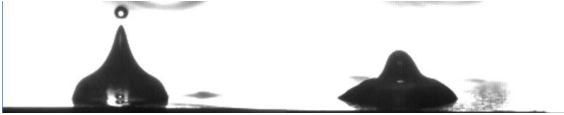
Figure 24. Satellite droplet separation success at low Weber number condition(left) and failed at high Weber condition(right)
