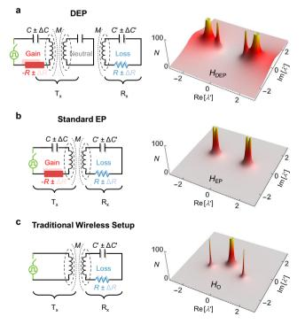
**Fig. 2** | **Pseudospectra of non-Hermitian circuits.** Transmitter–Receiver (Tx-Rx) architecture that implements a DEP (**a**), a standard EP (**b**), and a traditional near-field telemetry setup (coil antenna) without any EPs (**c**). The corresponding pseudospectra are plotted on the right panel.
