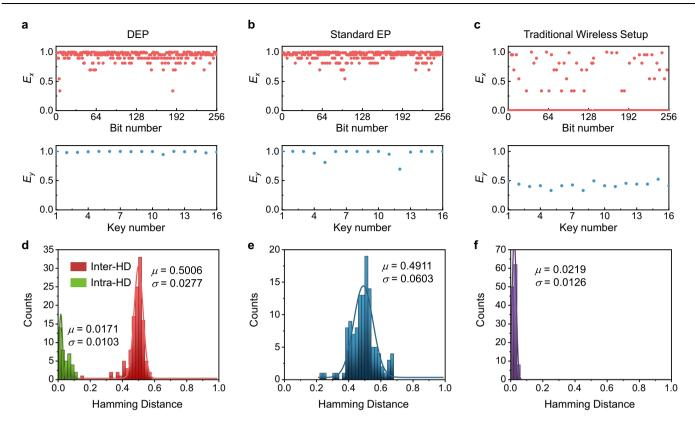
**Fig. 5** | **Statistical evaluation of PUFs.** Entropy  $(E_x, E_y)$  of the 256-bits PUF response from 16 manufactured PUF instances for the DEP-based (**a**), EP-based (**b**), and traditional RF PUF system (**c**) used for the identification application. **d**-**f** are similar to **a**-**c**, but for the inter-Hamming Distances (inter-HDs) histograms obtained from the
