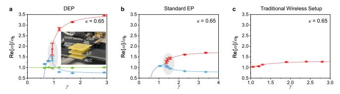
**Fig. 4** | **Experimental demonstration of high uncertainty near the DEP.** Theoretical (solid lines) and experimentally measured (points) eigenspectra for DEPs (**a**), standard EPs (**b**), and traditional telemetry setups (**c**), whose equivalent circuits
