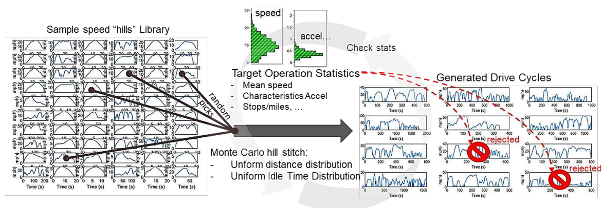
Figure 2. Monte Carlo approach to the generation of 2200 drive cycles for a delivery van application.
