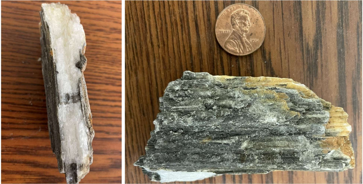
Sparitic veins with multiple slickensides on both sides of the surfaces. Layering on its surface suggests at least five episodes of movements
