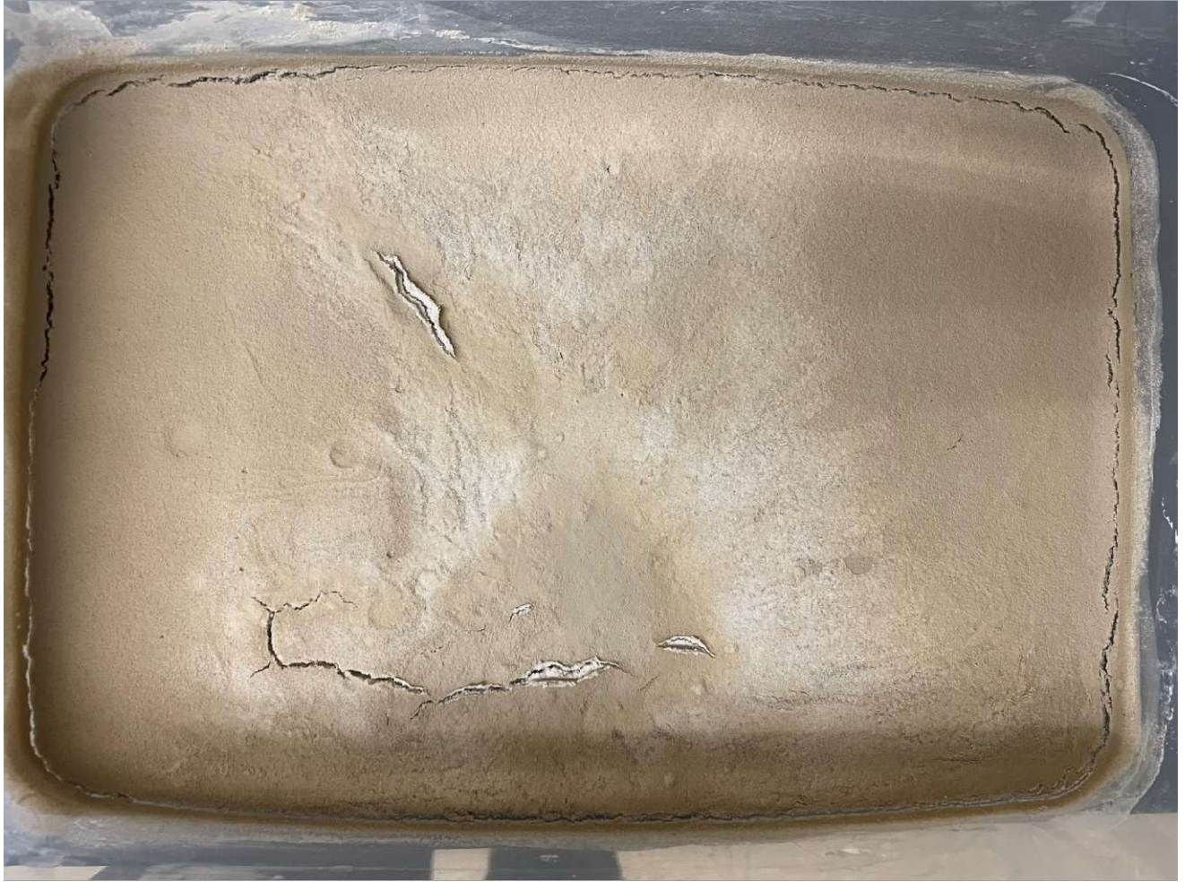
Cracks formed in 94% silica sand(500.98g) and 6% bentonite(30g). Only one continuous fracture formed on the center of the tray and it forms triple junctions with its branches.
