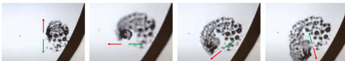
Figure 3-11. Asymmetrically loaded \text{MnO}_2 hybrid motor rapidly expelling bubbles (red arrow), propelling the motor in the opposite direction (green arrow) of bubble expulsion in 10% \text{H}_2\text{O}_2 and 30% \text{iPrOH} in water (table 3-2 entry 37).
