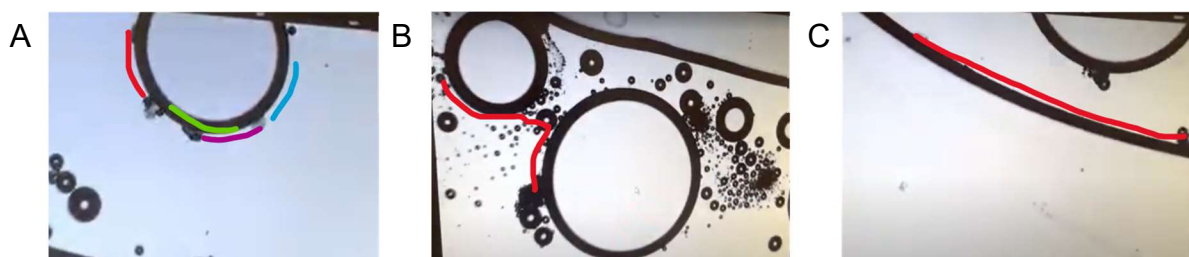
Figure 3-7. Micromotor propulsion at air-liquid interfaces. (A) Several 25 \mu\text{m} \text{MnO}_2 circular prints skating along the surface of an air bubble in 10% \text{H}_2\text{O}_2 and 60% EtOH in water (table 3-2 entry 54). (B) Motor skating along a bubble and then hopping to a neighboring bubble in 10% \text{H}_2\text{O}_2 and 30% EtOH in water (table 3-2 entry 52). (C) Motor skating along the boundary of the solvent in 10% \text{H}_2\text{O}_2 and 30% EtOH in water (table 3-2 entry 49). Motion over time is tracked using colored lines.
