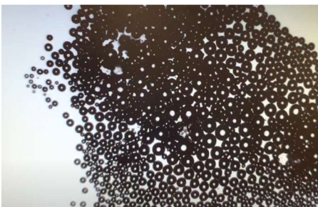
Figure 3-4. Motors in water with soap, 1% SDS and 3% H 2 O 2 . (Table 3-2 entry 62 in experimental methods section).
