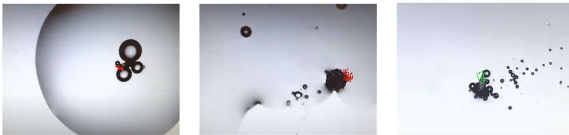
Figure 3-9. Wriggling motion of (A) \sim 100 \mu\text{m} motor in 3% \text{H}_2\text{O}_2 in ethanol (table 3-2 entry 43) and (B) \sim 100 \mu\text{m} motor in 3% \text{H}_2\text{O}_2 in water (table 3-2 entry 77). (C) \sim 150 \mu\text{m} cone shaped asymmetrically loaded motor in 10% \text{H}_2\text{O}_2 with 30% isopropanol in water (table 3-2 entry 31). Motion over time is tracked in red or green.
