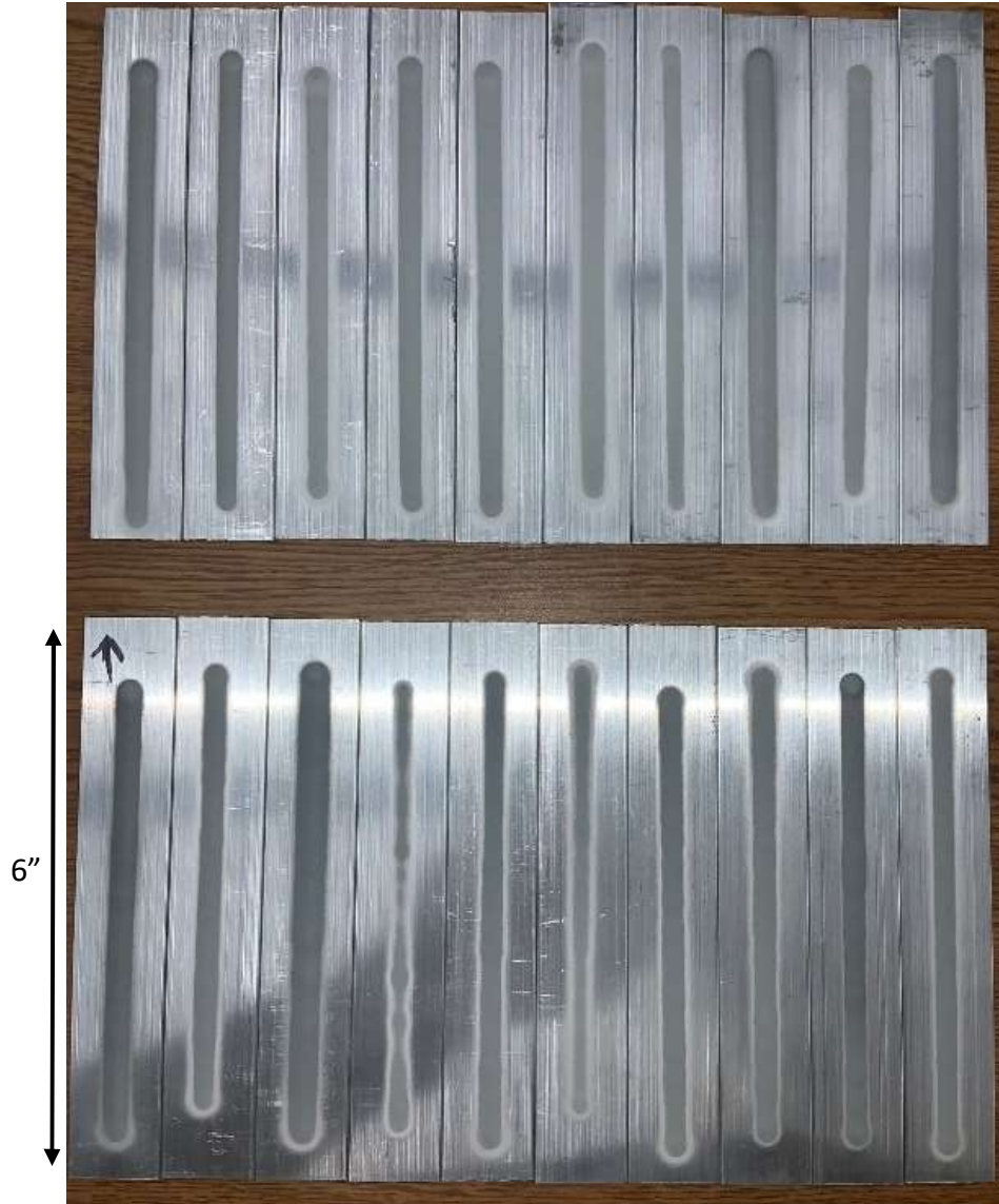
Figure 14: Zinc CS deposits in accordance with the experimental design to minimize statistical bias
