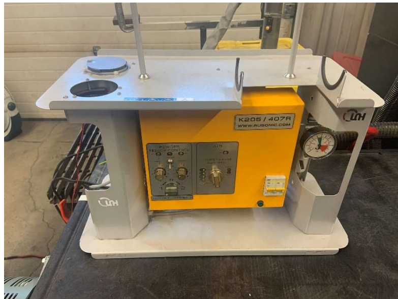
Figure 26: In-house RuSonic CS machine with separate feed hopper and heating element controlled through a variable transformer
