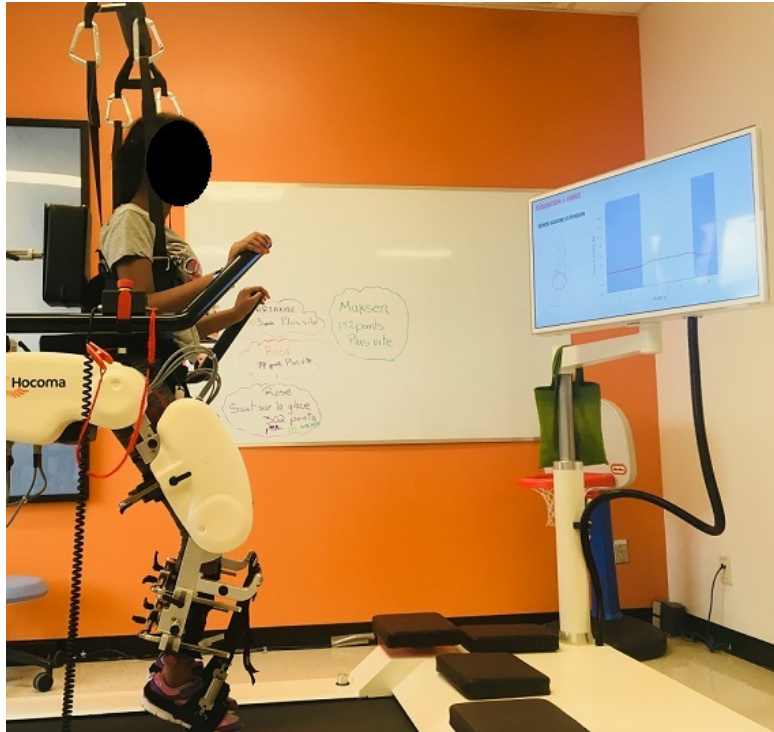
Figure 1: Subject installed in the position used for the MVIT measurement with the L-Force tool. The Lokomat is set to position control mode with preset fixed joint angles (hip 30° flexion, knee 45° flexion).
