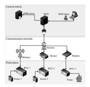
Figure 5. A typical SCADA Architecture A SCADA Testbed for Investigating Cyber Security Vulnerabilities in Critical Infrastructures (Tesfahun 2015)
