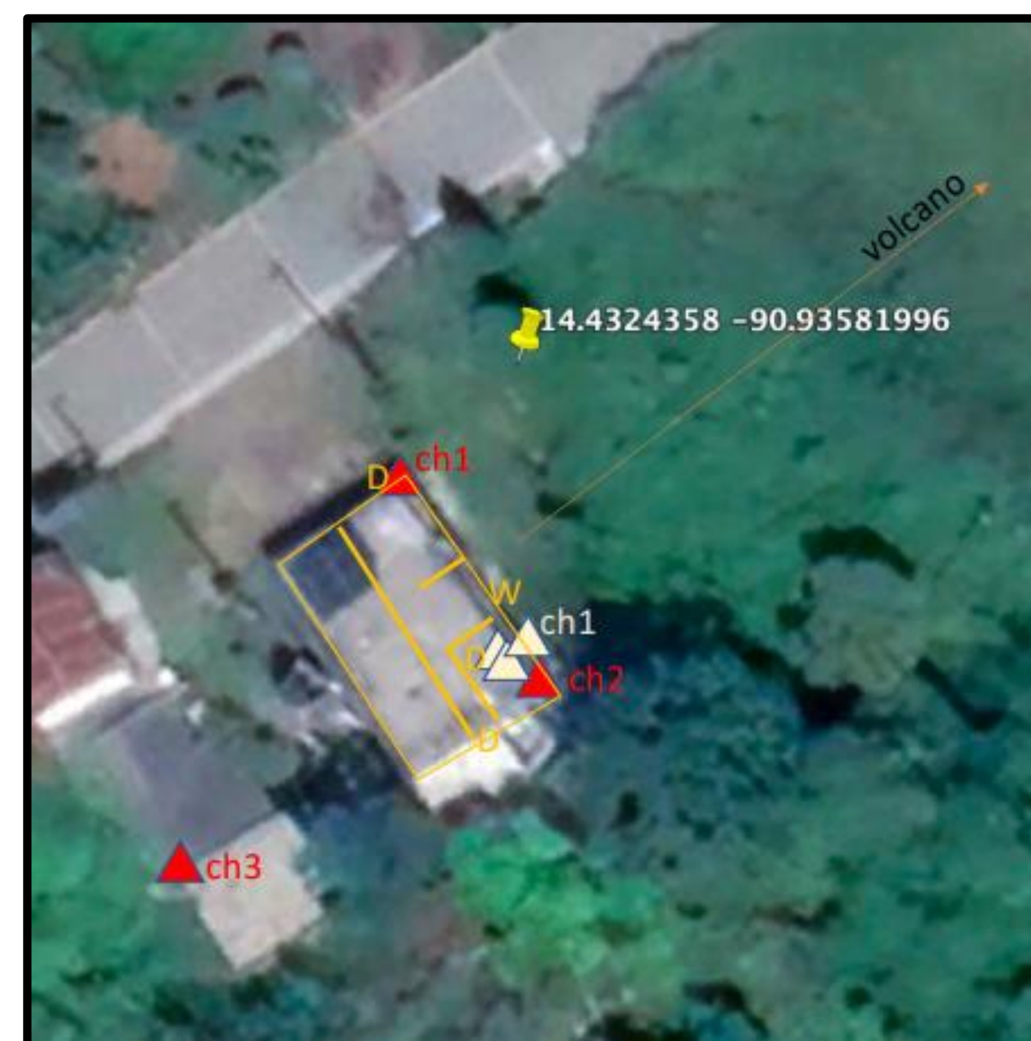
Figure 1: Google Earth (2022) Outside sensors in red, inside sensors in white; Fuego observatory briefly outlined in yellow (W denotes open window, D denotes closed doors)
