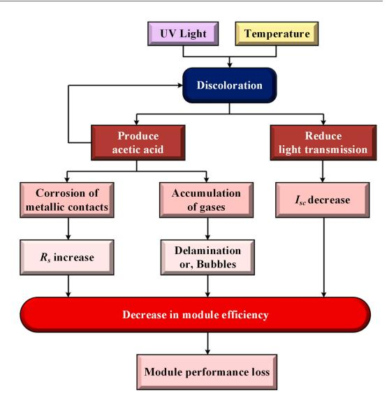
Figure 3. Flow chart of PV aging process through discoloration [69].
