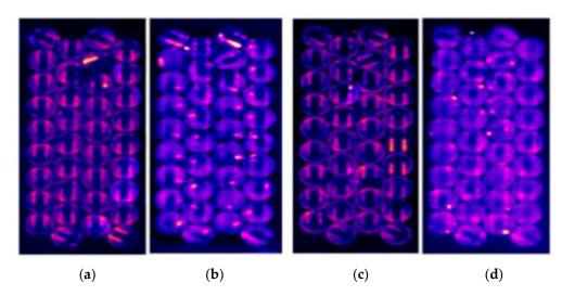
Figure 4. Temperature variation in discolored and non-discolored PV modules [69].
