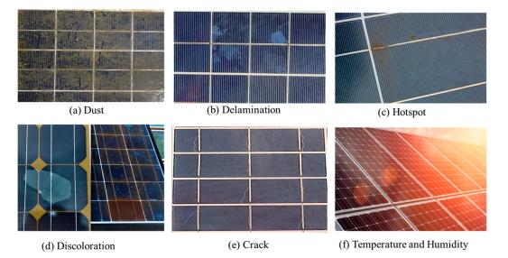
**Figure 1.** Key aging factors that affect the longevity of the PV module (this figure was developed from the original sample and experiments that were carried out in the laboratory).
