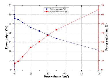
Figure 8. Reduction in PV output power due to the accumulation of dust panels.
