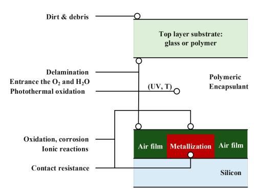
Figure 6. PV degradation process through delamination [89].
