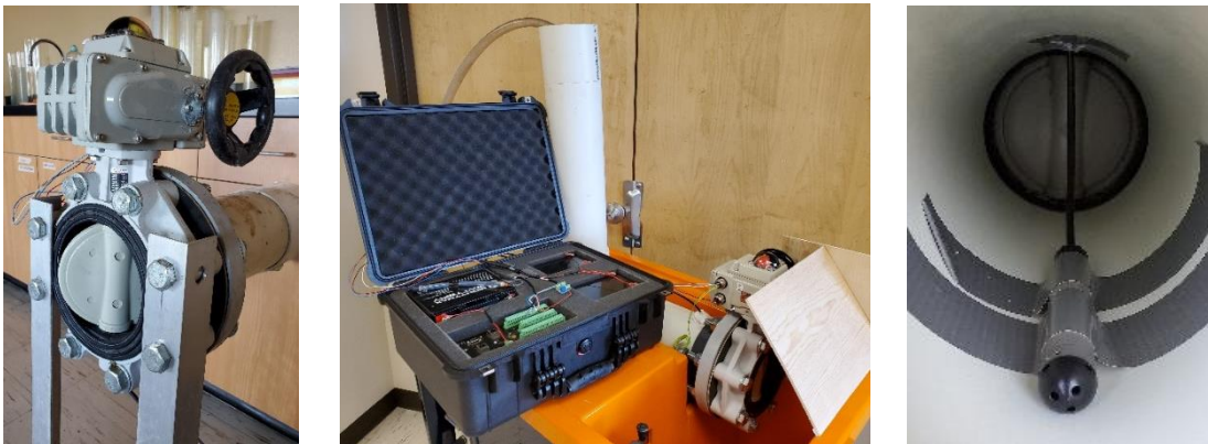
Figure A 4-1. Active control set-up in the laboratory. The figure on the left illustrates the activated valve connected to an underdrain and supported by aluminum legs; the picture in the center illustrates the testing apparatus of the activated valve in a hydraulic; the picture on the right illustrates the pressure transducer installed inside the 6-inch underdrain and shows the installation of the pressure transducer to measure water level within the underdrain and behind the butterfly valve.
