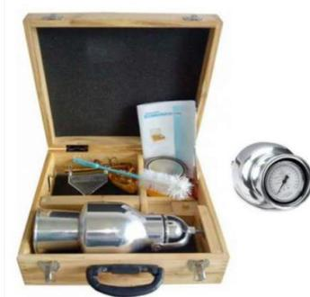
**Gambar 3.14** Alat Speedy Test
