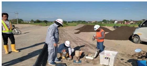
**Gambar 3.15** Pengoperasian Speedy Test
