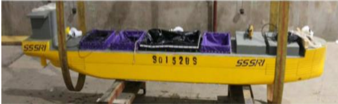
Gambar 3. 8 Model kapal open top container 800 TEUS
