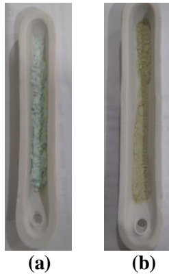
Gambar 4.3 (a) katalis \text{Mg}_{0,95}\text{Ni}_{0,05}\text{F}_2 sebelum kalsinasi (b) katalis \text{Mg}_{0,95}\text{Ni}_{0,05}\text{F}_2 sesudah kalsinasi
