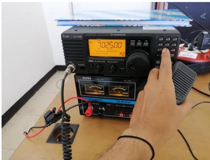
**Gambar 4.5** Pengecekan Kanal Melalui Rig HF *Transceiver*
