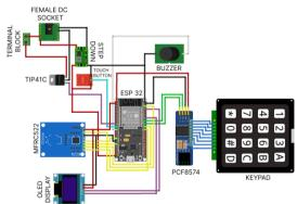
Figure 6. Diagram of smart door lock system
