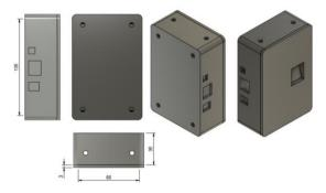
Figure 8. Design of PSU and touch sensor
