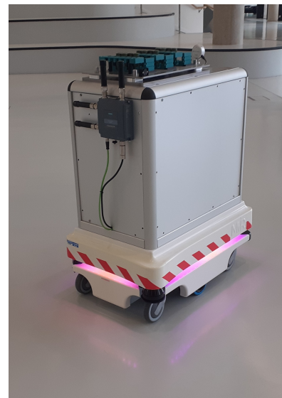
FIGURE 9. The completed 5G MiR100 AGV carrying a sub-assembly.
