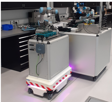
FIGURE 13. 5G AGV delivering an assembly to a robotic FMS station.
