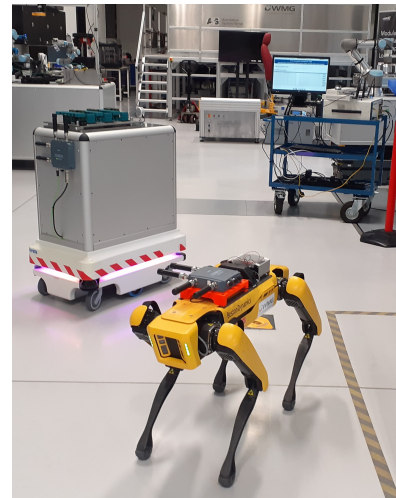
FIGURE 16. The 5G AGV testbed is operational and is being extended to other types of industrial mobile robots and manufacturing cells.
