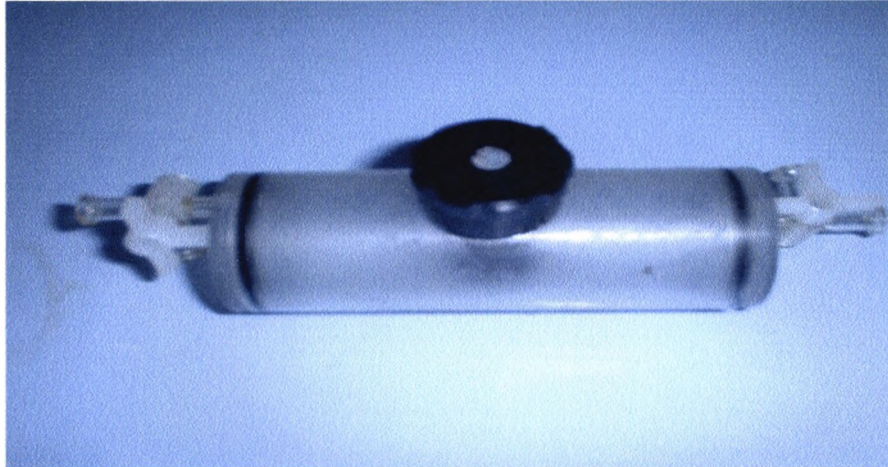
Figure 4.6. The sample holder used for the investigation of the effect of angle on T2^* . The black handle on the side allowed for a precise manual rotation of the sample within the syringe in accurate increments of 10 degrees.
