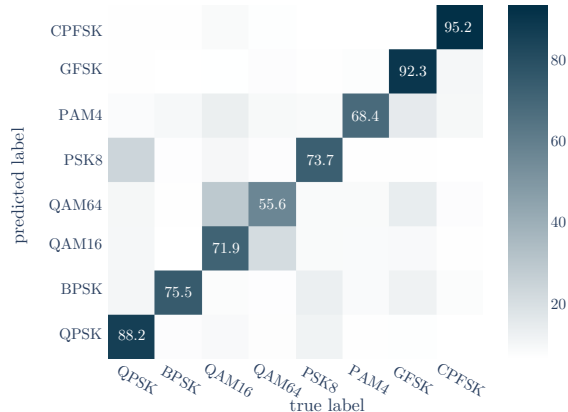
Fig. 4. Accuracy metrics for modulation classification with RFSoc in loopback.
