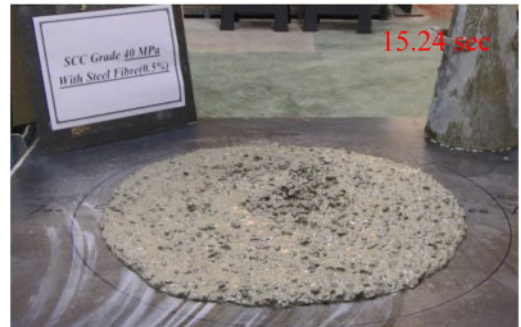
Figure 6. Experiment of slump flow test for SCSFRC (0.5%vol fibre).
