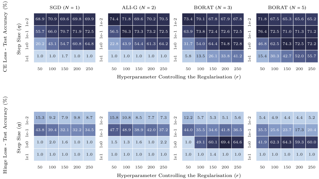
Figure 4.5: Comparison of SGD, ALI-G and BORAT’s robustness to hyperparameters when increasing N for the CE and SVM losses. Experiments are performed on the CIFAR-100 data set. Colour represents test performance, where darker colours correspond to higher values. For both losses, increasing N allows for higher learning rates to be used while still producing convergent behaviour. Additionally, for the CE loss and \eta \in \{1.0, 10.0\} larger N allows for a smaller r or greater levels of regularisation to be used. Consequently, increasing N improves the overall robustness to hyperparameters, while not sacrificing generalisation performance.
