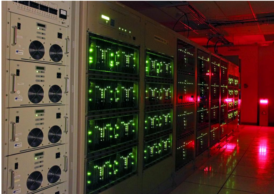
Figure 2.3: The ALMA 64-input Correlator used by the 12-m array. This is housed in the ALMA Array Operations Site Technical Building. Credit: ALMA (ESO/NAOJ/NRAO), S. Argandoña.
