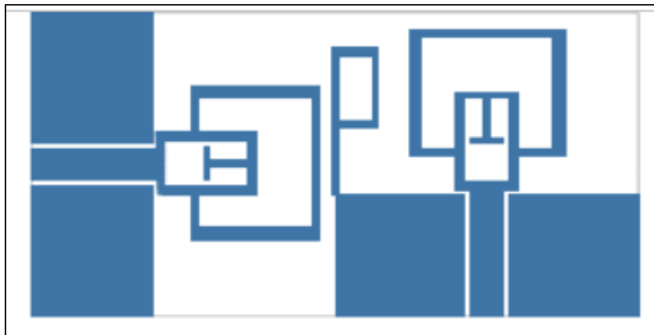
Figure 14: Design of two MIMO antenna placed vertically [49].
