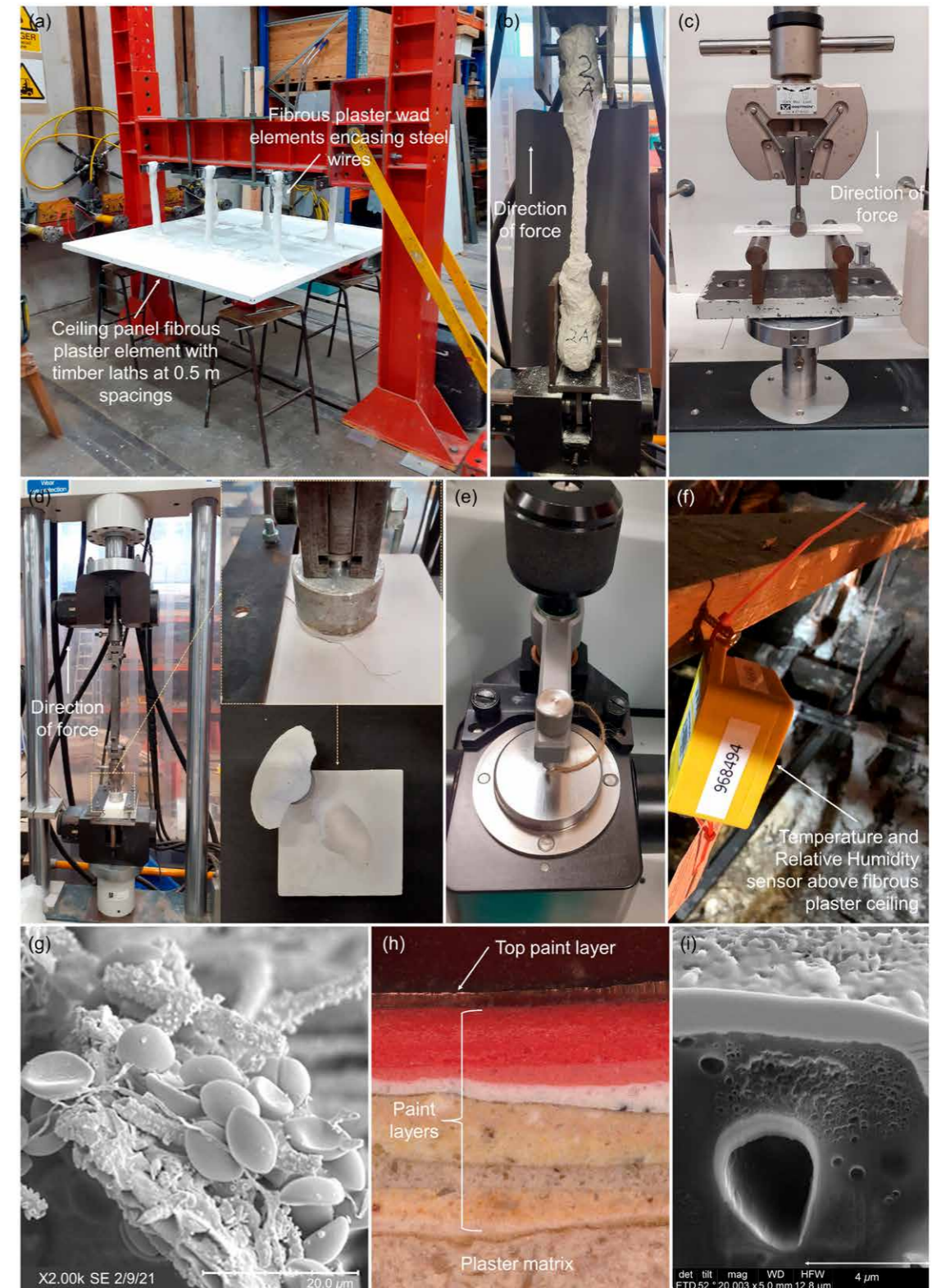
Figure 2: Selected images of fibrous plaster tests undertaken at the University of Bath, a) large scale 1.5 metre x 1.5 metre plaster ceiling panel with wads attached to supporting steel beams, b) Tensile testing of an individual wad element, c) Flexural tests of 6 millimetre thick rectangle fibrous plaster panels, d) Adhesion ‘pull-off’ tests rig and close-up images of cylinders representing repair materials applied to bases representing historic plaster material, e) Fourier-transform infrared spectroscopy using Attenuated Total Reflection characterisation of a hessian fibre bundle, f) Environmental sensor on the topside of a theatre ceiling, g) scanning electron microscope image showing suspected fungal spores in a historic fibrous plaster sample, h) Optical microscopic image of paint layers applied to fibrous plaster matrix, and i) Focused Ion Beam image of a single hessian fibre cross section. All images by the authors.
