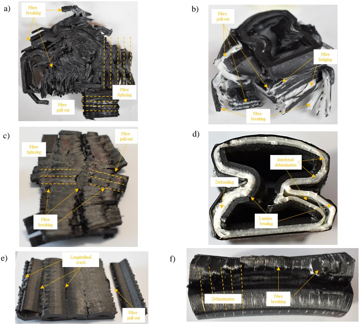
Figure 9. Post-impacted profiles. a) Fibre splaying and breaking on CDA, b) Fibre bridging and breaking on GDA, c) Fibre breaking and pull-out on CDR, d) Interhead delamination and lamina bending on GDR, e) Longitudinal crack on CDR f) Interlayer delamination and fibre breaking on GDR.
