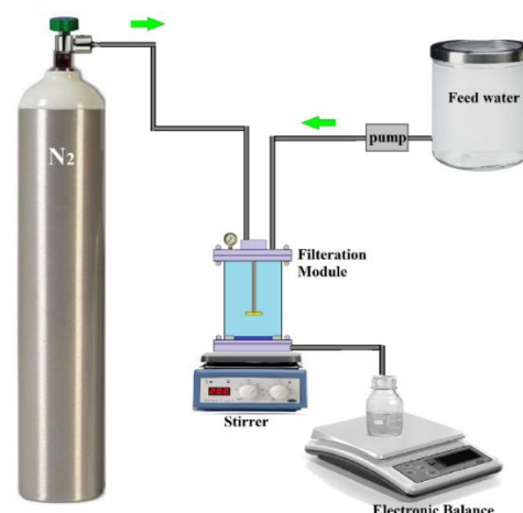
Fig. 1 The schematic of the used dead-end filtration.
