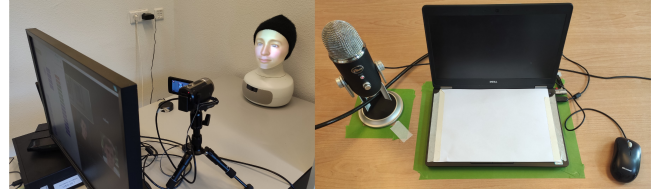
Figure 1: Setup at the office (robot’s side, left) and the school (child’s side, right).
