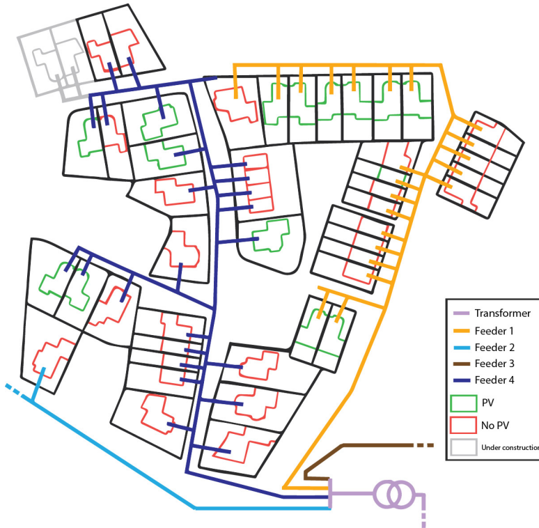
Figure 2.3: A layout of the electricity cables in De Veldegge in 2019. Created based on the image provided in [120].
