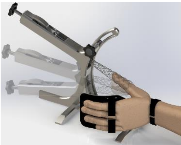
FIGURE 13: ARTICULATING DISTRATOR OF THE THUMB MCPJ, FINAL DESIGN.
