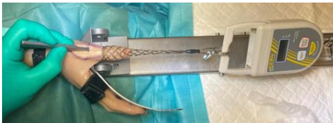
FIGURE 4: MEASURING THE CREATED SPACE DURING THE DISTRACTION OF THE THUMB MCPJ.
