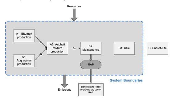
Figure 1. System boundaries of the LCA study.
