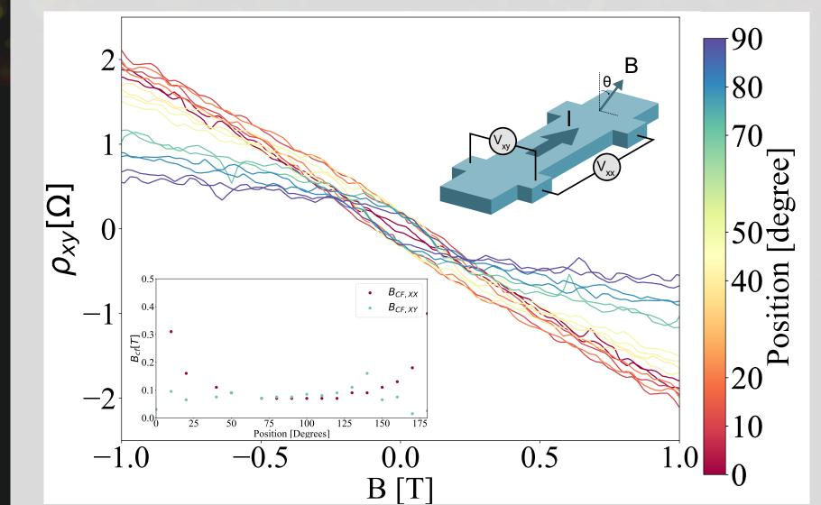
For a varying direction of the B-field, an hysteresis appears in the Hall resistivity as well.
