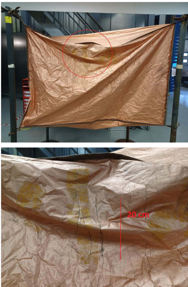
Fig. 6 Wrinkles and cracks in Kassel cloth due to wear (1) (picture from outside VIRC).
