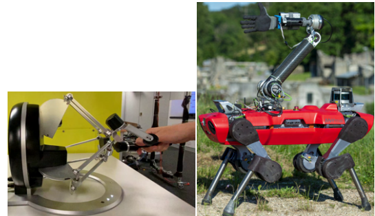
Fig. 1: Experimental setup with Omega6 as haptic device at the master side ( left ) and the ANYmal C platform equipped with a robotic arm at the slave side ( right ).
