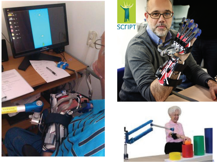
Figure 13.2 Upper extremity exercise system including robotic support for the hand functioning, gravity compensation and individually tailored video games (Scriptproject.eu).
