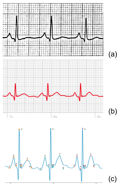
Figure 3. Example of lead II of a 12-lead ECG (a), AW-II PDF extract (b), and the extracted digital AW-II SVG signal (c) derived from the same patient. In the digital tracing (c), for each of the three heartbeats, eight points are indicated, from which the four amplitudes and three durations are then automatically determined. The eight points are defined as follows: 1. Onset P-wave, 2. Amplitude P-wave, 3. Onset QRS-complex, 4. Amplitude QRS-complex, 5. End QRS-complex, 6. Amplitude ST-segment, 7. Amplitude T-wave, 8. End T-wave.
